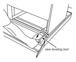
Make sure you lower BOTH REAR ROLLERS. There are two adjusting nuts, one for each roller, at both the front bottom corners of the cooker.
